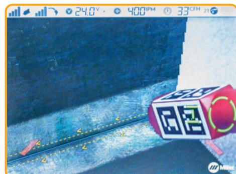
Actual proximity and interaction data is processed by the system via specially coded devices and coupons
