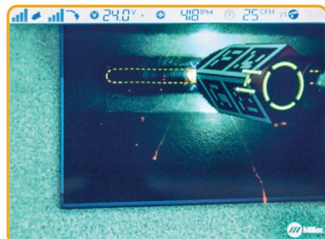
During a simulated weld sequence, visual graphical aids guide user to achieve adherence to parameters.
