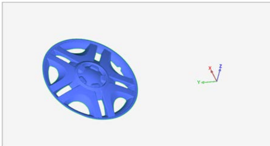
Figure 18: Object before alignment—random coordinate system.
