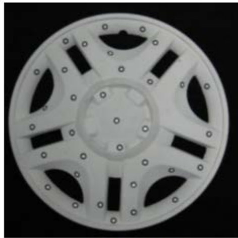
Figure 37: Representation of targets application.
