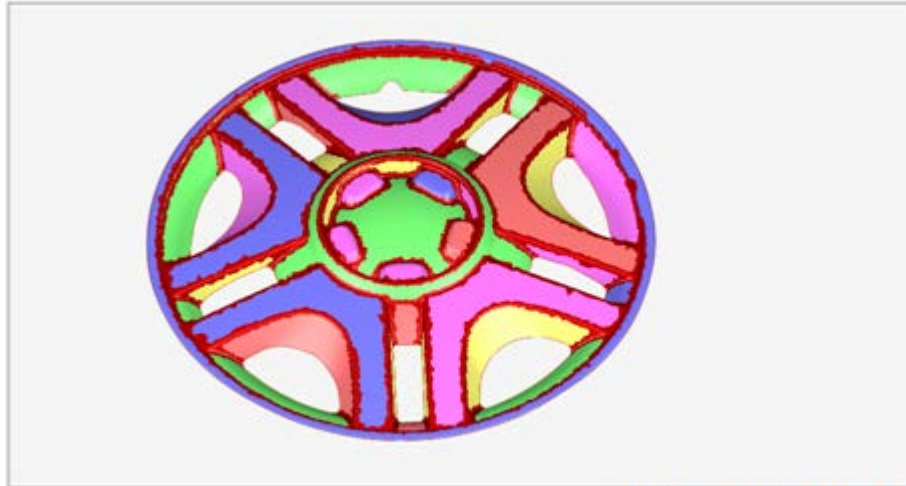
Figure 17: Representation of object into different regions/shapes (segmentation).
