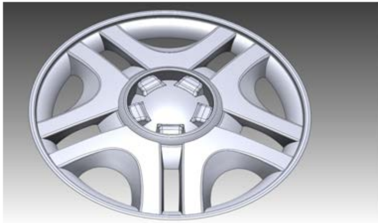
Figure 20: Creation of one entity and repeated circular pattern to create the entire object.
