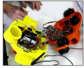
Top shell (yellow) and bottom shell (orange) are both FDM parts.
