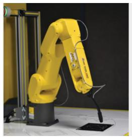
**Fenceless Arc Mate -** FANUC ARCMATE 50*i*D/7L education cart cell for ArcTool (AT) operations. ArcTorch with embedded laser pointer and welding coupons simulate the welding process.
