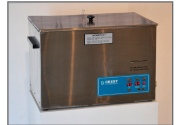
Supports on the parts are dissolved away in a tank filled with an alkaline-based solution.
