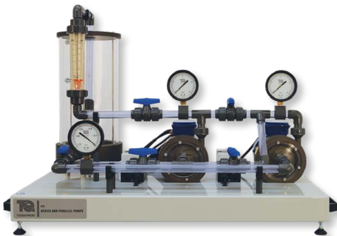
SERIES AND PARALLEL PUMPS (H52)
