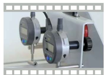
UNSYMMETRICAL BENDING AND SHEAR CENTRE EXPERIMENT
